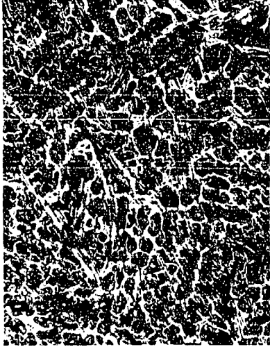
Alloy M-8. 0.429% Cr., 1.91% Si. Structure as cast. Nitric acid etched. 75 X.
